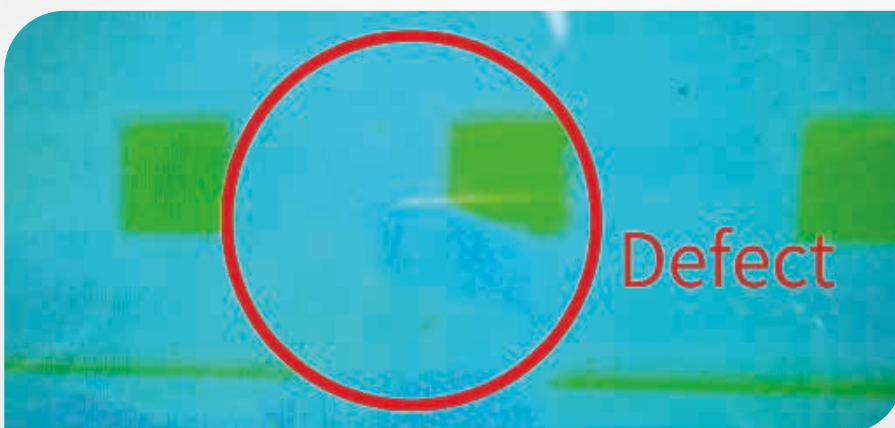
Inspect Defects from Silicon Side Wafer
