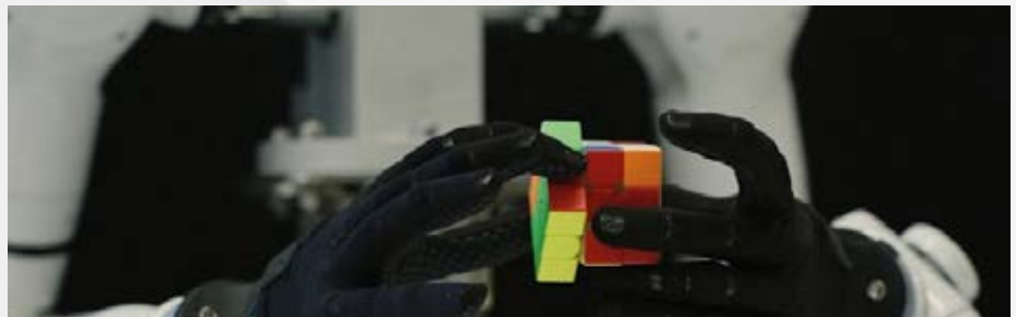
Genesis AI's dexterous robotic hands manipulate a Rubik's Cube using continuous in-air manipulation requiring coordinated, high-speed reasoning and precise wrist control, at the company's facility in San Carlos, California, U.S, June 9, 2026. Genesis AI/Handout Via REUTERS
