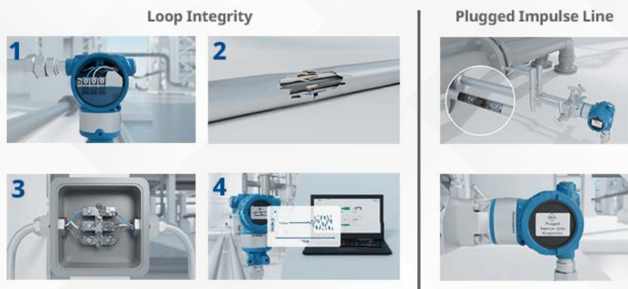
Figure: Loop Integrity and Plugged Impulse Line Diagnostics Troubleshooting on the Rosemount™ 3051 Pressure Transmitter
