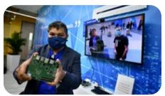
Mr Varun Chatterji, co-founder and chief software architect of Seventh Sense, holding a ZCU104 board running a Resnet 50 Facial Recognition Model in real time. ST PHOTO: LIM YAOHUI
