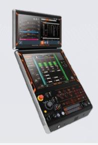
Graphical user interface enhancements, an optional second monitor and operation panel enhancements to support other new SMOOTH TECHNOLOGY solutions, including Solid MAZATROL, SMOOTH Ai Spindle, and Ai Thermal Shield.
