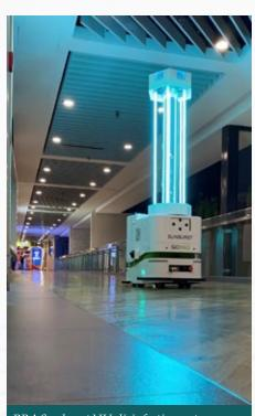
PBA Sunburst UV-disinfecting autonomous mobile robot emits powerful UV-C rays which can eradicate viruses. [Photo credits to PBA Group and Frasers Property]
