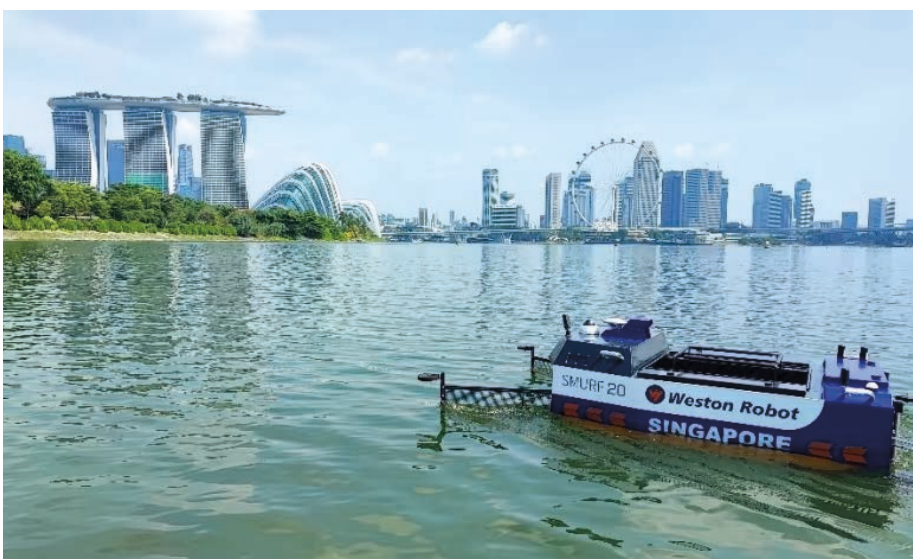
A 5G-enabled electric unmanned surface vessel for river cleaning and inspection. (Photo: Weston Robot)
